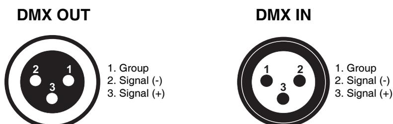
If you are using controllers with this occupation, you can connect the DMX-output of the controller directly
